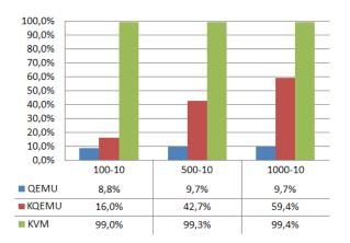
Figure 8. QEMU, KQEMU, KVM performance using WDT benchmark (Increasing ratio of userspace operations)
