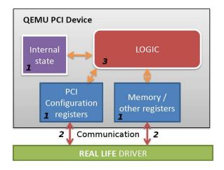
Figure 5. Development process using QEMU
