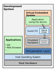
Figure 2. Virtual platform system schema
