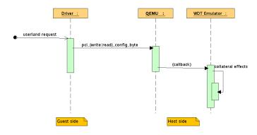
Figure 6. Execution flow of a request to WDT emulator
