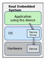
Figure 1. Real embedded system schema
